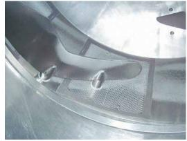
After coating, the inside of pan is very clean compared to other enteric coating agents. You can save time for cleaning.
