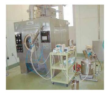
Since the nozzle clogging was found to be caused by the strong binding of the polymer and plasticizer, this technique was developed. The key of this method is to spray the two components separately. Using this technique, you don't have the clogging problem, and you don't need to chill the dispersion as in the regular method. As the polymer can be applied in greater concentrations than the regular method, you can achieve shorter processing time.
